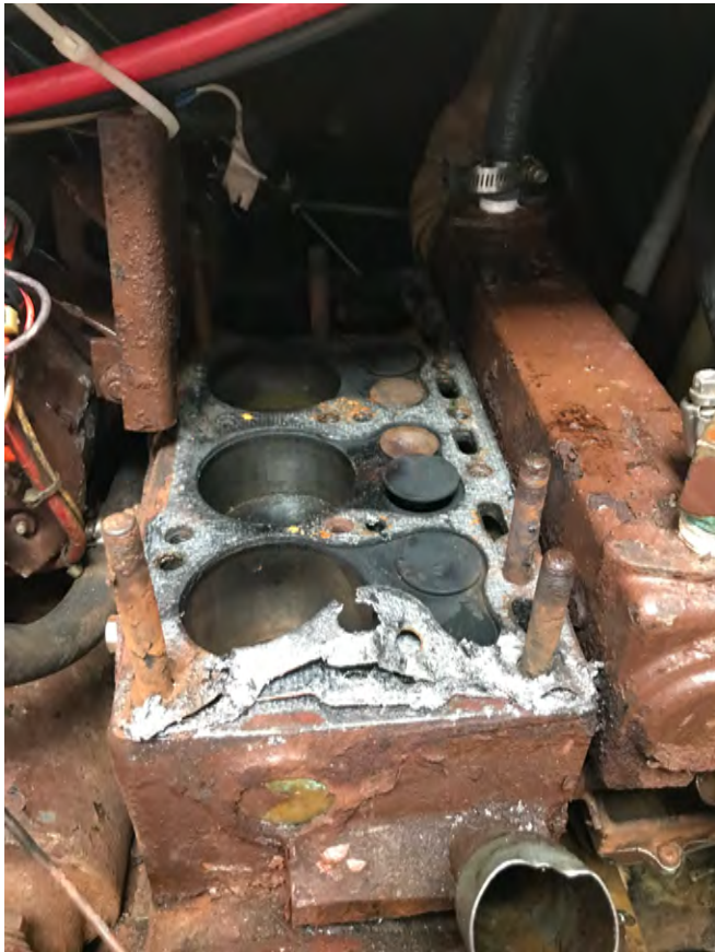
Cylinder Block after Head removal and in process of being cleaned - Six studs remain in block. Piston and valve heads and cylinders appear in good condition
