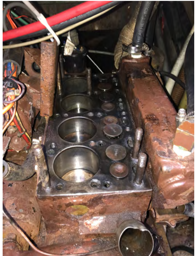
Cylinder Block after Head removal and in process of being cleaned - Six studs remain in block. Piston and valve heads and cylinders appear in good condition
