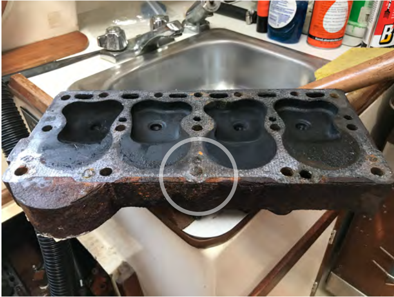
Old Cylinder Head Removed - Stud #8 (circled) broken off in head
