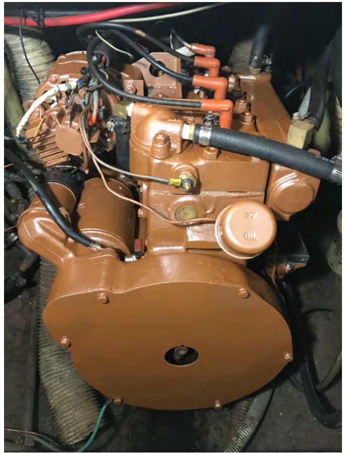
Final reassembly - note the nuts were also painted to prevent rust
