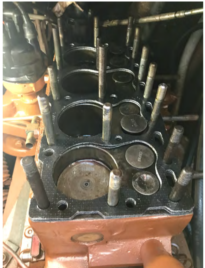
After final cleaning, two head gaskets placed before cylinder head installation
