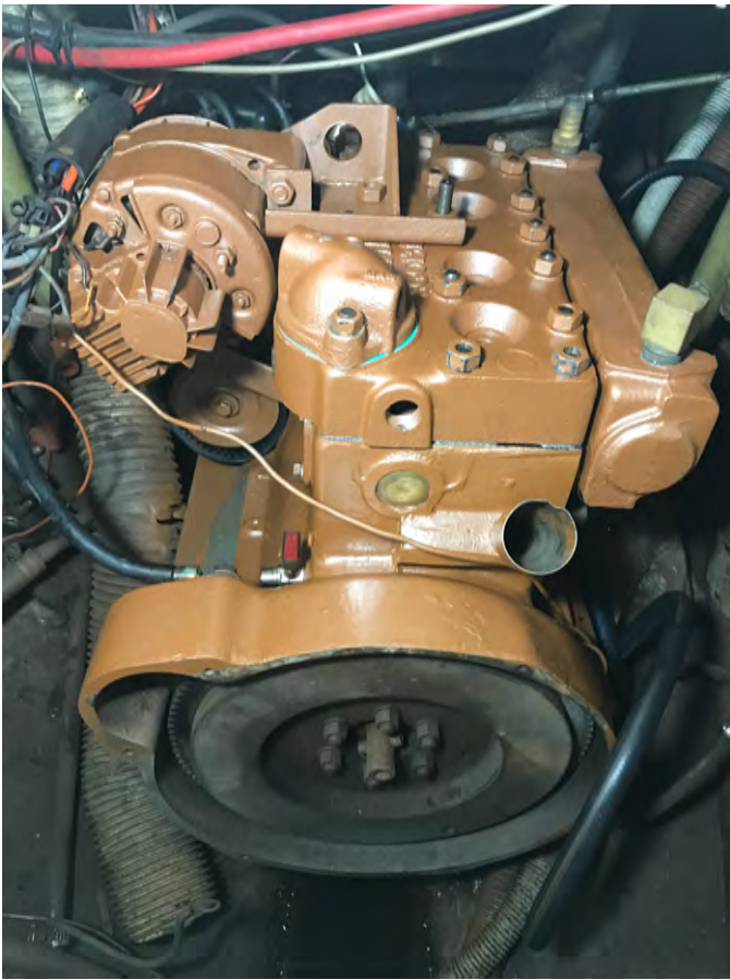
Engine block preservation completed, head installed and tightened as per manual (25, 30, and 35 ft-lbs of torque)
