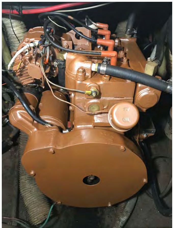
Engine with all painted comonents reassembled
