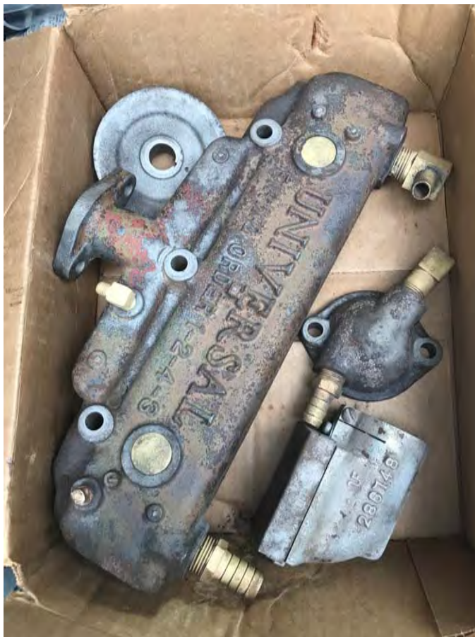
Components after sandblasting
