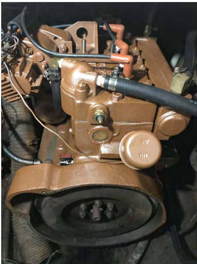
Engine reassembled without Flywheel Cover and Starter Motor
