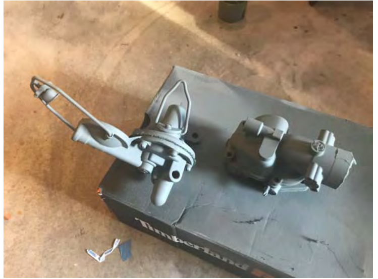
Fuel Pump Body with priming coat
