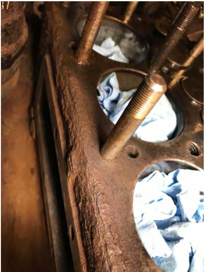
Close up of excessive corrosion on starboard side of engine block
