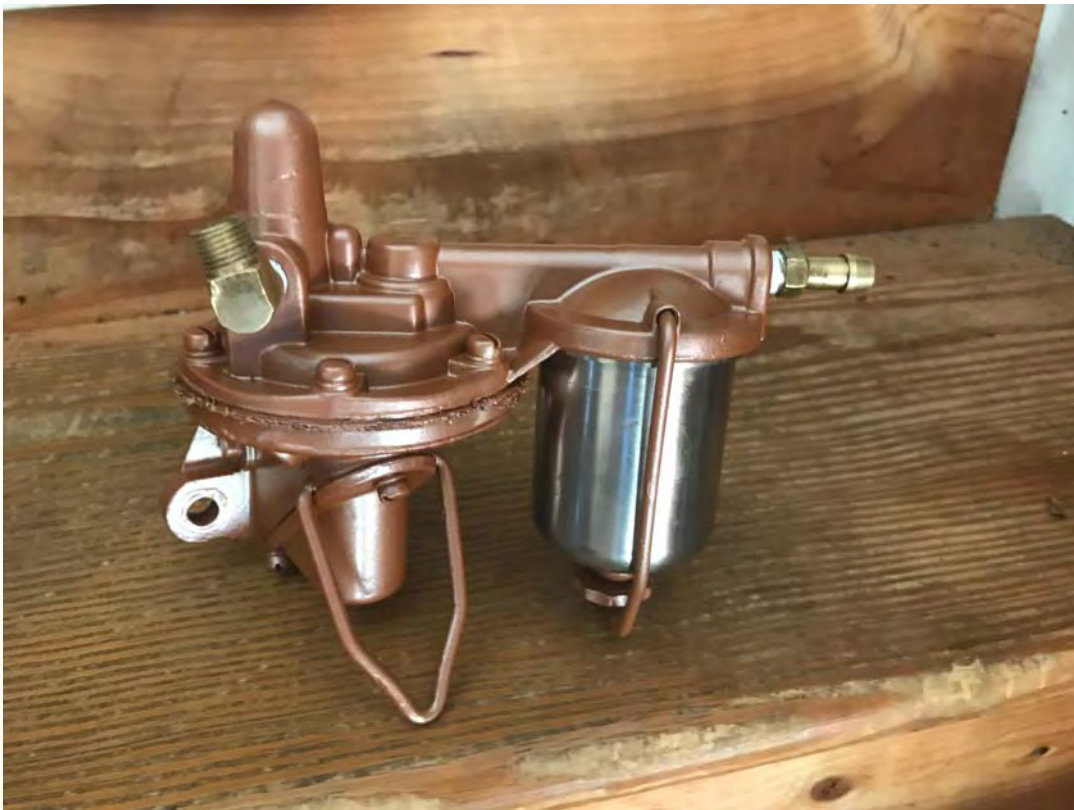
Finished Fuel Pump and Sediment Bowl
