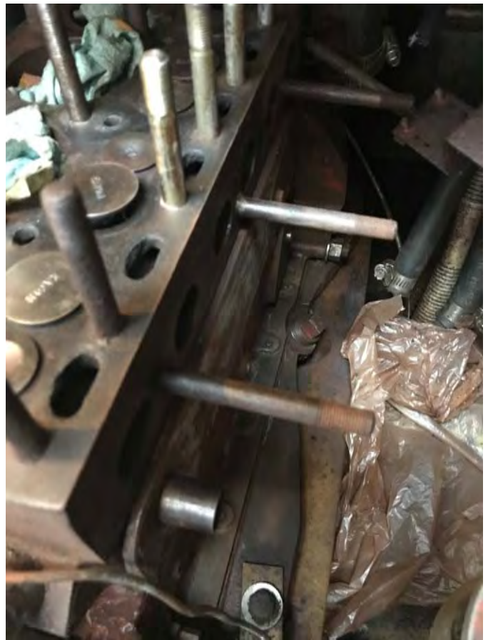
Final engine (port side) descaling and cleaning
