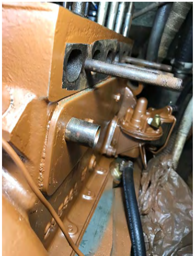
Engine (port side) painted and components reassembled
