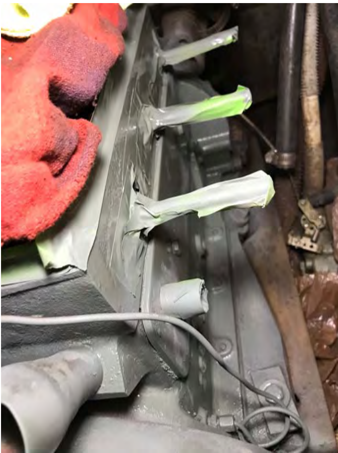
Primer coat applied to port side of engine
