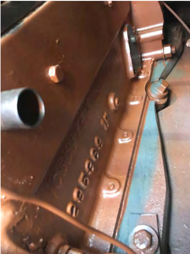
Finishing coat on port side of engine
