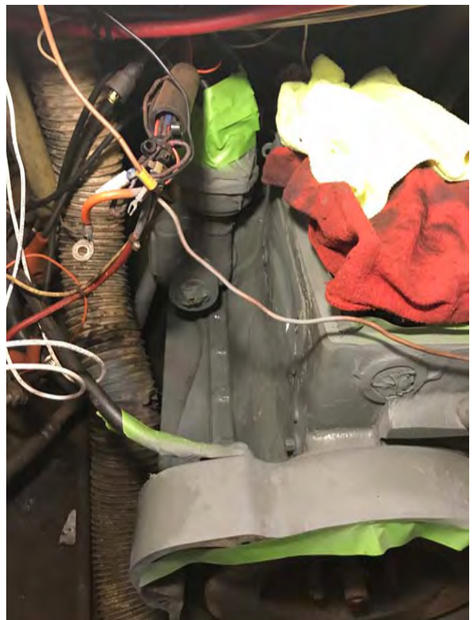
Primer Coat applied to engine (starboard side)
