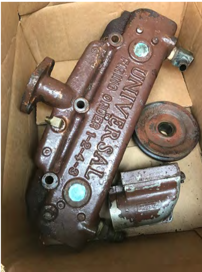
Manifold, Alternator Pulley, and Spark Arrester before sandblasting and cleaning
