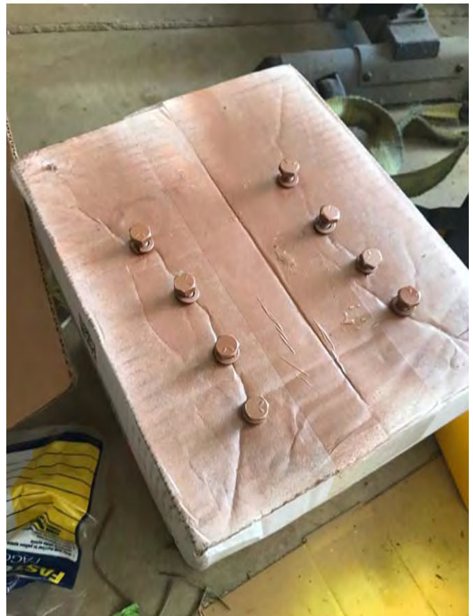
Painting bolts for Jacket Water Plate
