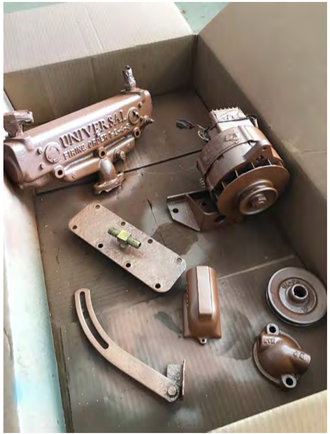
Setting components to dry for at least 24 hours
