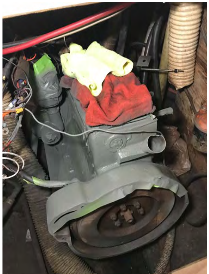
Final primer coat applied to engine
