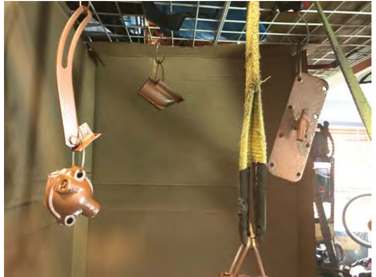
Coating alternator bracket, thermostat housing, jacket water plate, and flame arrester
