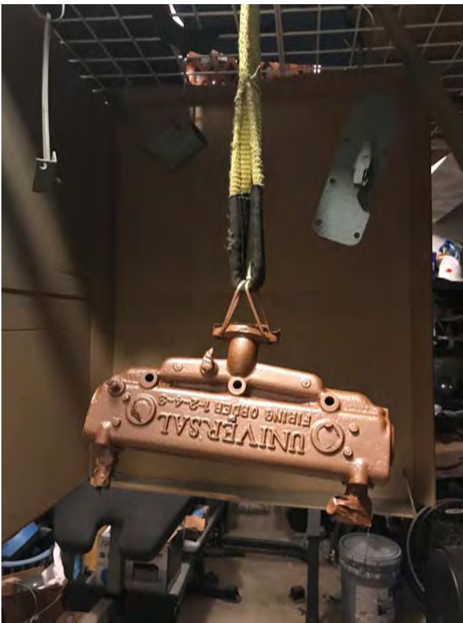
Manifold coated with high temperature paint, other pieces painted with self-etching primer
