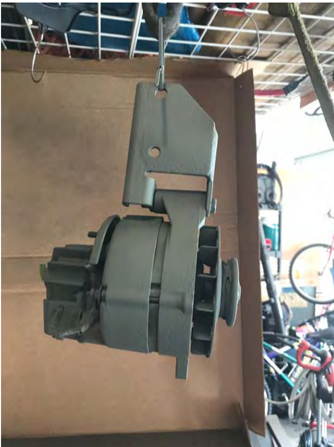
Spray painting alternator with self-etching primer (passages to windings closed with tape)
