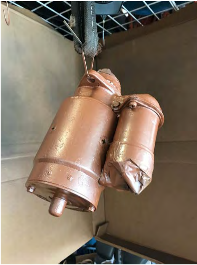
High temperature spray paint on Starter Motor/Solenoid
