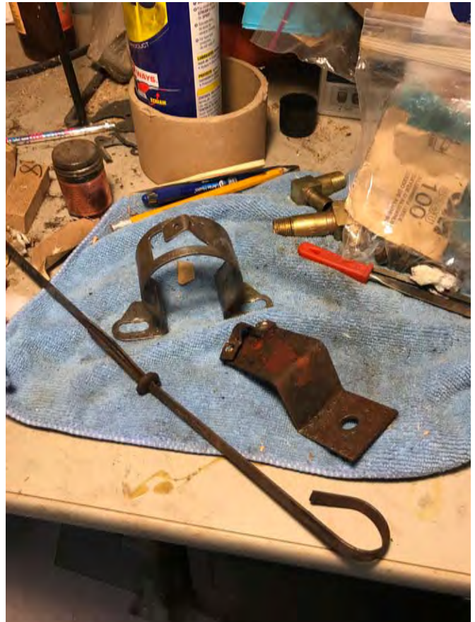
Ignition Coil Bracket, Dipstick, and Throttle Bracket before cleaning
