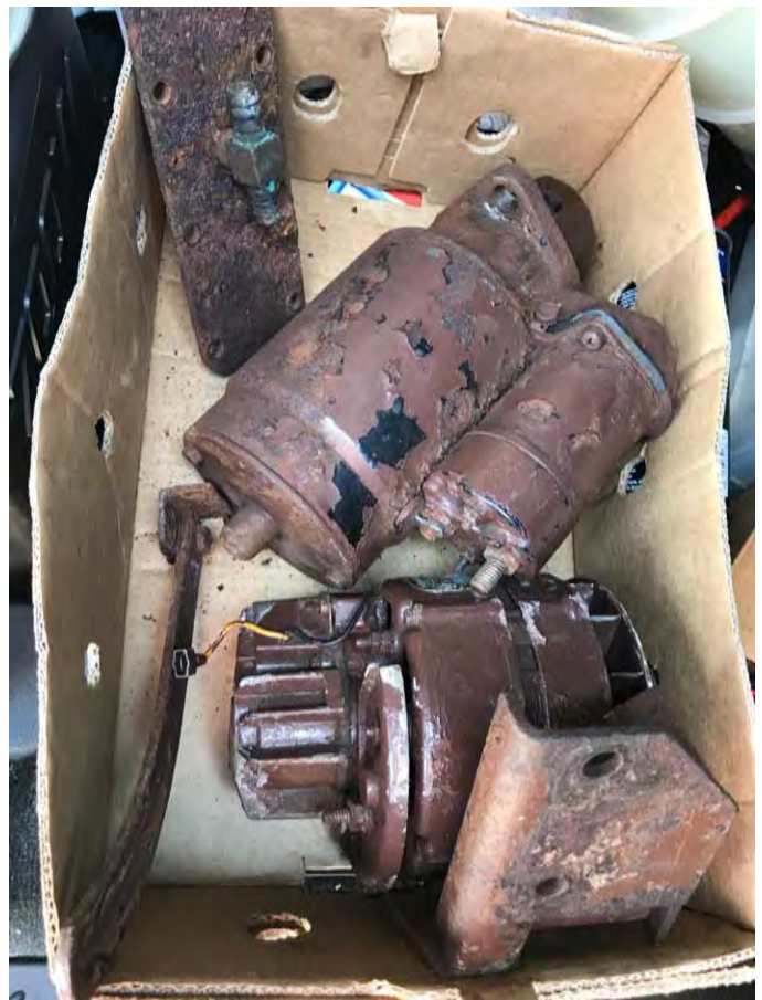
Jacket Water Plate, Starter Motor, Alternator and Alternator Support Bracket before
