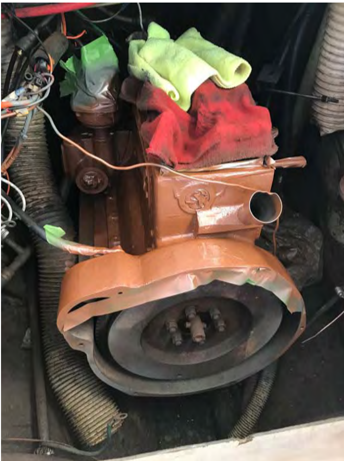
Applying "antique copper" high temperature spray paint to engine
