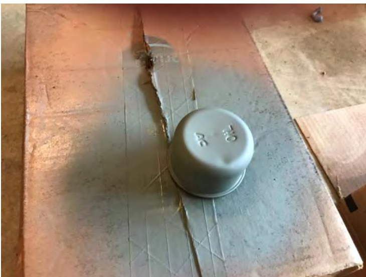
Oil Breather/Fill Cap with primer coat
