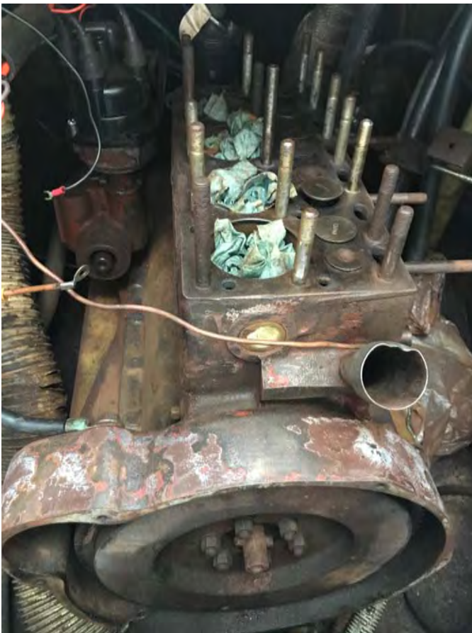
Final engine descaling and cleaning before self-etching primer coat
